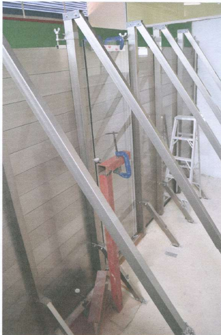
Figure 3 Leakage measurement section and Horizontal measurement points
