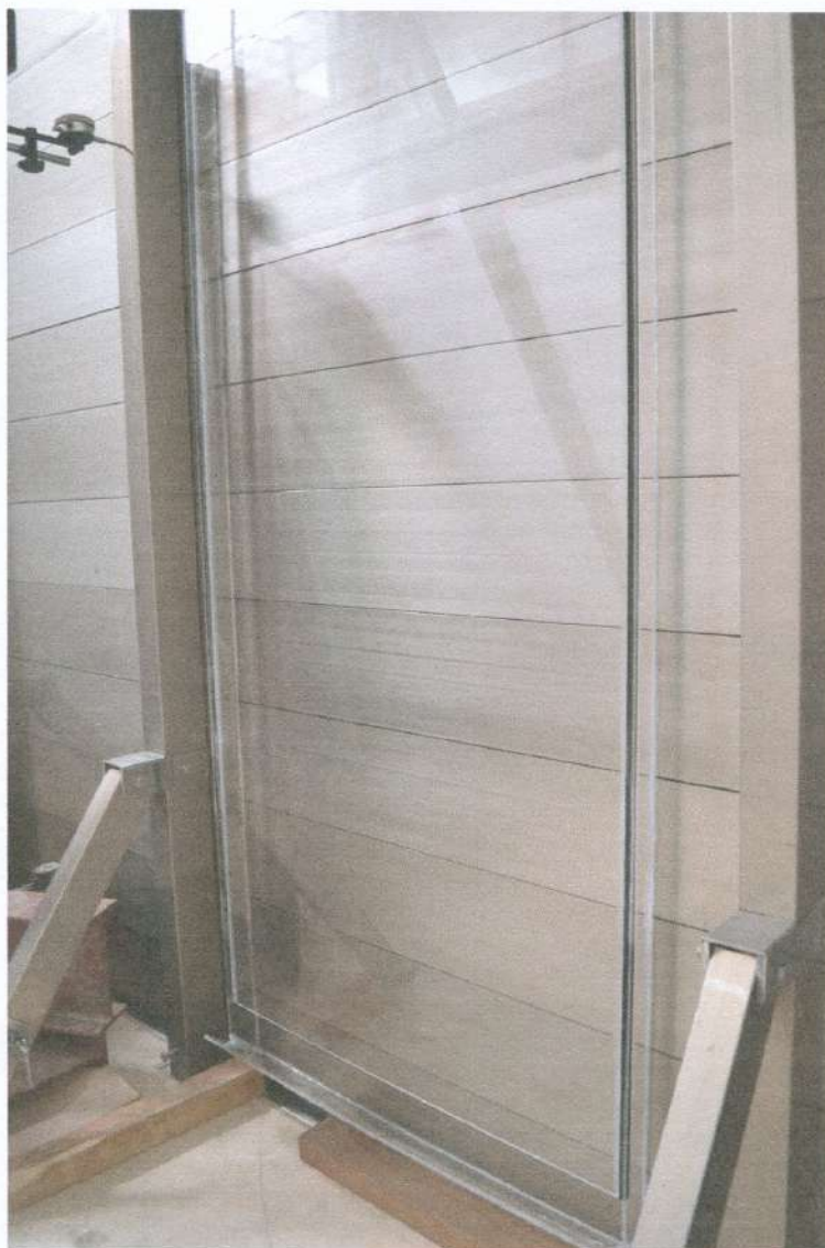
Figure 4 Leakage measurement section
